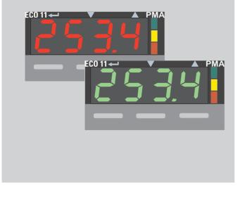
Indicator, signaller, or two-point controller Output sense selectable direct/inverse Accurate control behaviour with 250 ms scanning cycle High-precision universal input Auto/manual switchover w/W2 from front panel Up to three switching outputs (control output & alarms) Output function selectable as control or alarm RS 485 with Modbus RTU protocol Front panel protection mode IP 66
